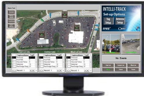
**Intelli-Track** is a scalable, PC-based, system designed specifically to provide RFID asset tracking with our technology partner TRES (Transponder and Reader Engineered Systems).
