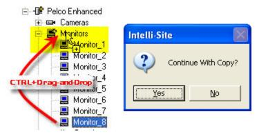
Note: The position of the Monitor node in the tree corresponds to the physical monitor output number on the Switcher: For Example: Monitor\_6 corresponds to the 6<sup>th</sup> video output on the switcher.
