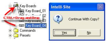
Note: The position of the Keyboard node in the tree corresponds to the physical Keyboard output number on the Switcher: For Example: Keyboard\_4 corresponds to the 4<sup>th</sup> keyboard on the switcher.
