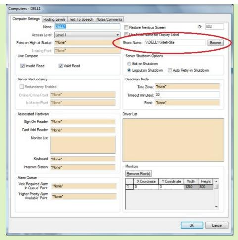
• Right click on the "Computers" node, select "Add Node and Edit..." Type in the name for the computer that will run the Workstation remotely. Click <Ok>.
