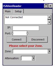
The Setup tab has a status box, IP address, Port, Connect, Disconnect buttons, Zone list, and Attenuation.
