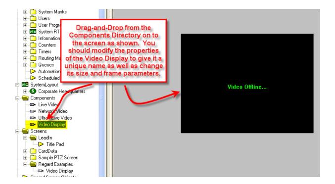
1. Create a control Screen Object (a button or icon) that directs a video channel (Camera) to the Video Display. The Action for any Axis command is always SendCommand, and the Target may be any Subnode in the Axis RTU. In the following example, we are sending live video stream (Camera) to the Video Display Object that we created in the previous step.
