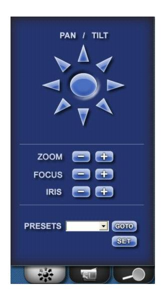
a. Pan/Tilt arrows- Clicking and holding the left-mouse button on an arrow will move the camera in the corresponding direction. Releasing the mouse button will stop the movement.
