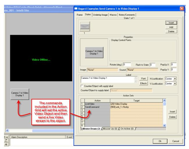
3. In Run Mode select the button (mouse-down, single left-click). The resultant display should be live streaming video to the Video Display Object:
