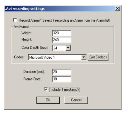
**'Record Alarm?'-** Select this check box if recording an alarm retrieved and selected in the 'Alarm List' at the bottom of the tab. Leave the checkbox unselected if recording video from the camera selected in the 'Camera' drop-down list at the top using the 'Goto' date/time fields.
