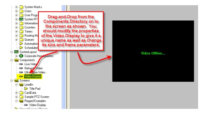
2. Create a control Screen Object (a button or icon) that directs a video channel (Camera) to the Video Display. The Action for any Milestone command is always SendCommand, and the Target may be any Subnode in the Milestone RTU. In the following example we are sending live video stream (Camera) to the Video Display Object that we created in the previous step.
