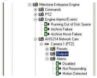
NOTE: Any Event buttons or Generic Events setup in the Engine must be manually added under the 'Engine Alarms/Events' node. This will allow the Event(s) to be reported on when using the Milestone Driver under Driver Service. To create a new Event, right-click on the 'Engine Alarms/Events' node and select 'Add Node'. The 'Address' field must contain the exact name of the Event in order for the Event to be found in the project tree:
