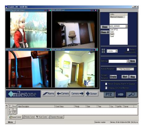
• Double click on any video feed. (For our example were using camera 1) This will enlarge the video to fill the area currently occupied by the n\*n channel view. Double click to return.
