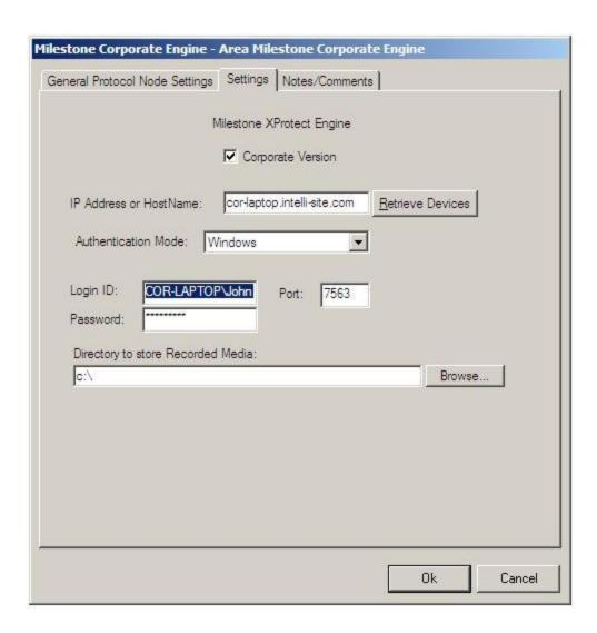
When all fields have been filled out. Select the 'Retrieve Devices' button. This will connect to the Engine and Auto create tree nodes for:
