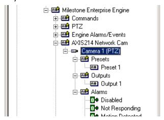
6. PTZ Command Nodes ('Tilt Up', 'Pan Right', etc.) can be used can also be used as the target of a SendCommand action to execute the given PTZF command. Commands are located here:
