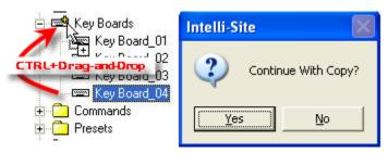
Note: The position of the Keyboard node in the tree corresponds to the physical Keyboard output number on the Switcher: For Example: Keyboard\_4 corresponds to the 4<sup>th</sup> keyboard on the switcher.
