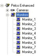
When the PEL node is initially added to the tree, the Monitors Node is pre-populated with 8 Monitors. This node can accommodate Monitors 1 through 254. To add a monitor:
